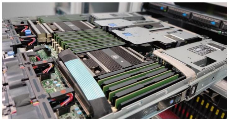
A candidate HLT node for Run 3, equipped with two AMD Milan 64-core CPUs and two NVIDIA Tesla T4 GPUs. Credit: CERN)
